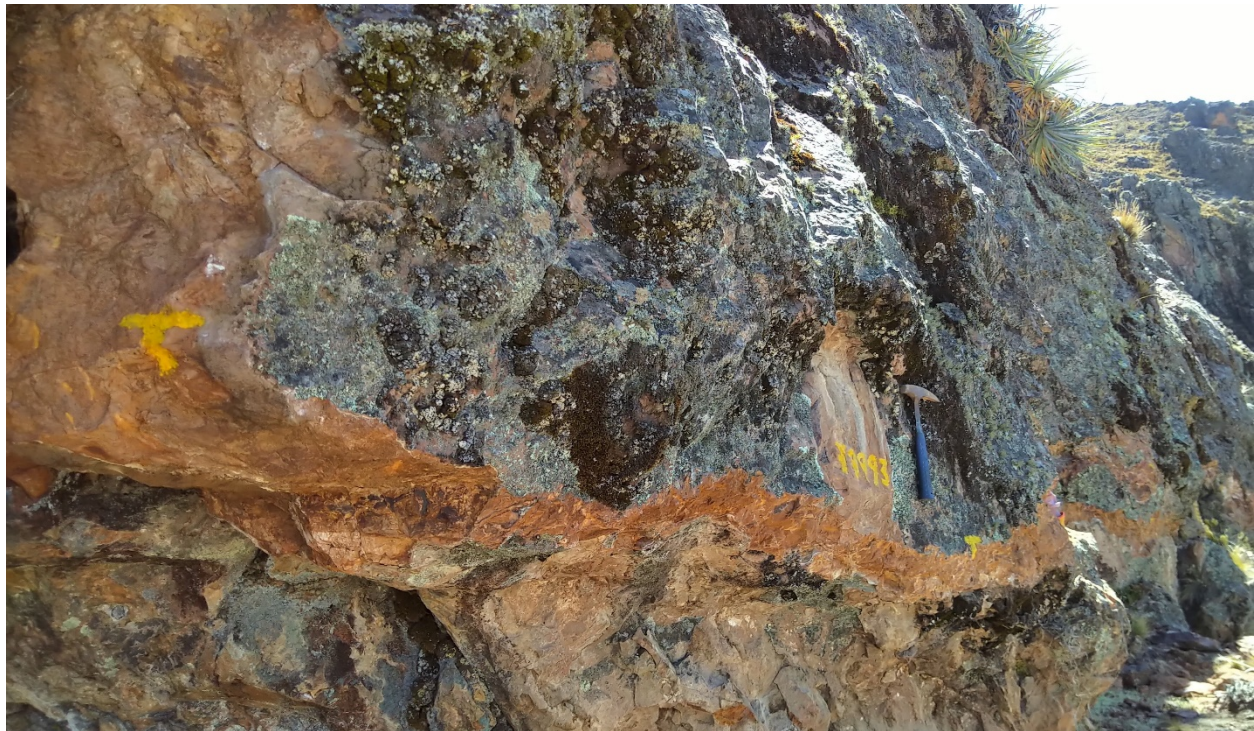
Figure 34. Original composite channel sample by Pucara, Cascada Diatreme. QP duplicate sample #621 (2 meter channel): 0.125 g/t Au
