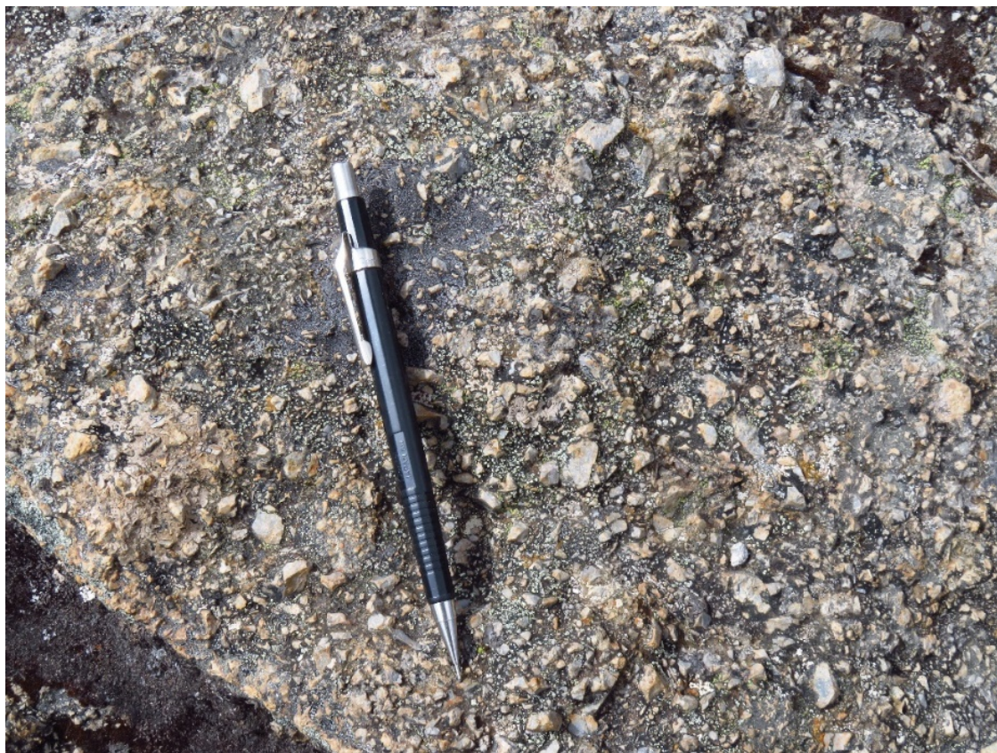
Figure 12. Typical finer-grained breccia texture of stratiform portions of the Central Diatreme with small, angular to sub-angular silicified clasts in a granular silica matrix.
